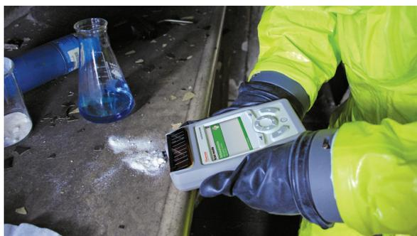
The Thermo Scientific FirstDefender RM instrument is a rugged Raman spectrometer for rapid, accurate identification of unknown chemicals directly in the field. At 1.8 pounds (800g), the FirstDefender RM analyzer includes a large, vivid display for ease of use in bulky protective gear and can be easily transported into a hazard zone.
