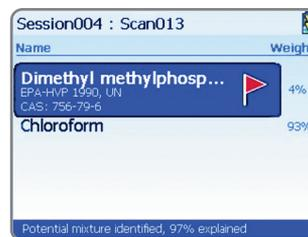
**Color-coded results require no user interpretation and provide rich content for faster, more informed decision making. Patented algorithms enable automatic mixture analysis, shown as a blue result, and tagged items are clearly highlighted on the result screen.**
